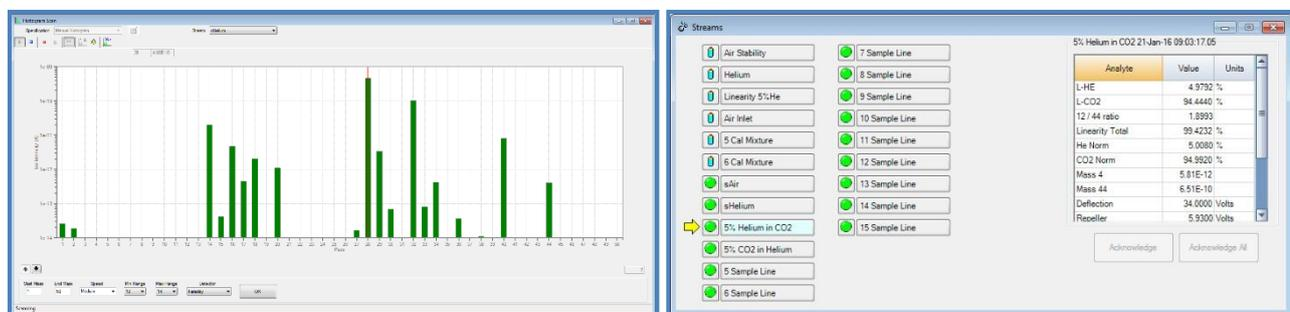
Many other data display forms are included in the standard GasWorks package including the “Scan” and “Streams View” forms shown above. The Streams View is particularly useful when the analyzer is used for environmental monitoring. Each sample stream is provided with a green/red LED style indicator and a button that is used to display
