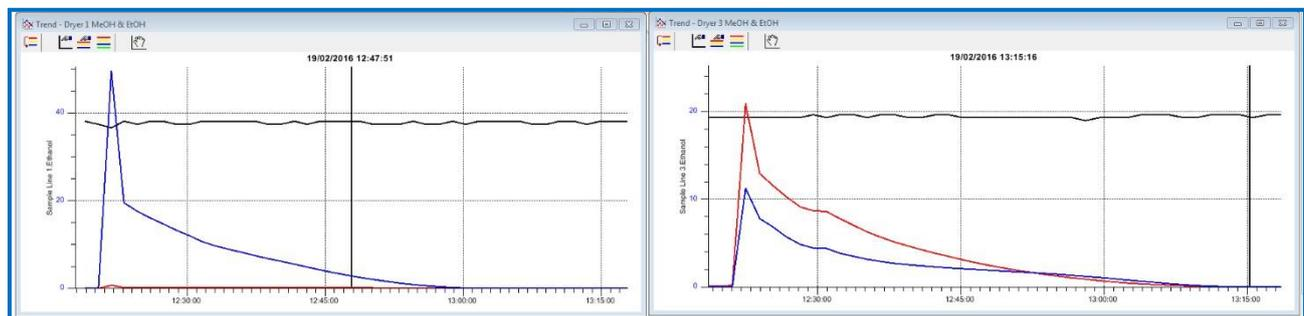
Each new trend form is configured using a set-up wizard which provides easy component and stream selection, axis configuration (log mode, linear mode, manual & automatic dynamic range, time, etc.) and trace color. Where a complex set of axes is required to present both logarithmic and linear plots on a single form then multiple y-axes are supported. Each form can be positioned and sized to make the best use of the available display area.
